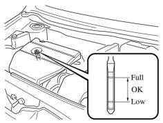
5. Pull it out again and examine the level. It's OK between MIN and MAX. But if it's near or below MIN, add enough oil to bring the level to MAX.
